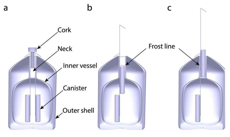
The anatomy of a LN Dewar with the canisters (a) in the storage position, (b) using recommended practices to access a canister, and (c) using common poor handling practices are shown. Note that the top of the canister is below the frost line in b and above the frost line in c.
