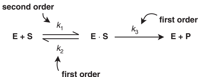
Figure 8-3 The Simplest Enzyme Mechanism
