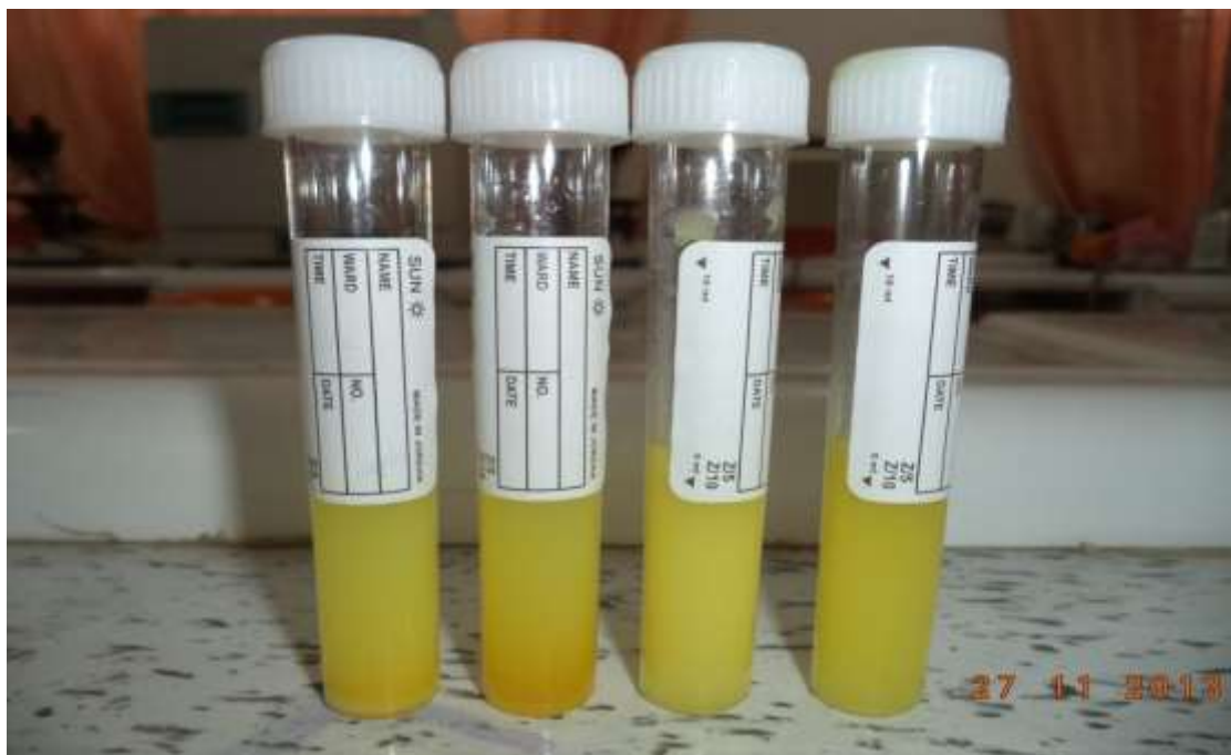
Fig- 7- Chloride test: Yellow colour indicating increase in chloride %.
